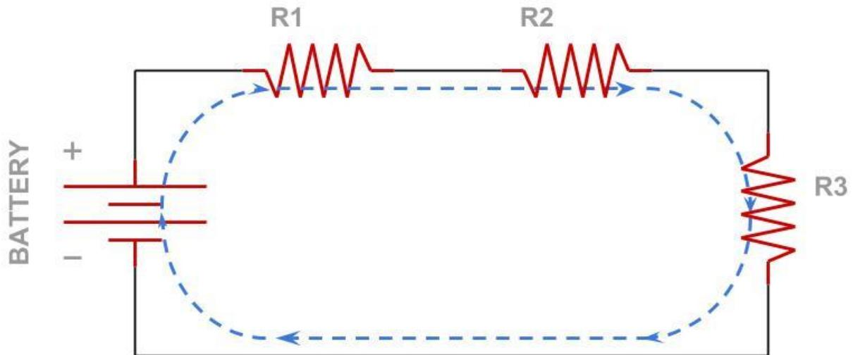
There's only one way for the current to flow in the series circuit. Current starts at the (+) end of the battery and flows through components before returning to the (-) end of the battery. Note that the current is constant through each component and the battery.
