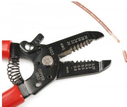
Although a knife would also strip the wires, it might also damage them by nicking the metal or cutting into it. Using a knife to strip wire is also really dangerous! The knife can easily slip and cause wicked injuries.
