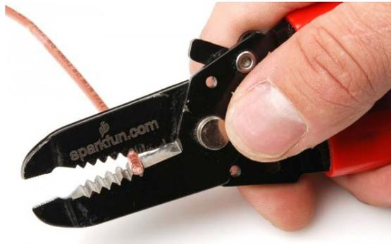
By simply squeezing the handles together about  $\frac{1}{4}$ " (or the desired length) from the end of the wire, using the correct notch on the tool, and then twisting the tool slightly, the insulation will be cut free.
