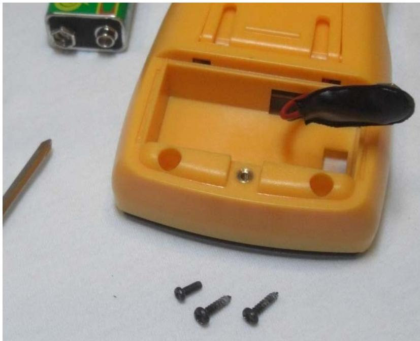
Remove the screws on the back of the multi-meter and locate the fuse(s) on the inside. Here should be a spare fuse in the meter. (It's a good idea to replace this if it used).
