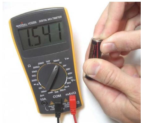
Checking Batteries: AAA, AA, C, and D batteries are nominally 1.5 V. Fresh batteries are about 1.6 V, and they lose voltage as they get used. Batteries with less than 1.4 volts are dead. 9 V batteries are made of six 1.5 Volt batteries in series, and a fresh 9V battery will show over 9 volts. Less than 8 volts can be considered dead.
