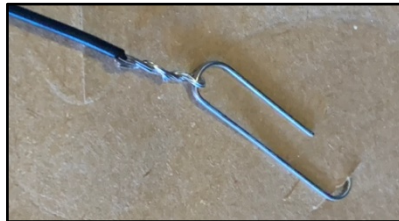
F) Paper clip on back with wire that connects to the LED (-) end
