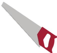
**Hand saws** come in a range of sizes and styles. There are many different kinds of tooth used for different types of cuts and materials. In general, small teeth are used for metal, large teeth for wood. Important concerns for drilling:
