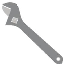
**Wrenches** are a metal tool that are typically used to tighten and loosen nuts, bolts, screws and pipes. The wide variety of wrenches includes adjustable and fixed size flat wrenches as well as ratcheting socket wrenches. Nut drivers combine a screwdriver handle with a socket head, and are convenient tools for turning nuts and bolts
