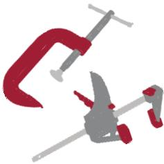
**Clamps** are portable device used to position parts while fixing them together. Clamps have two parallel surfaces to secure to part, and often one or both surfaces have angles that pivot or rotate to fit the surfaces of the part. Common types are C-clamps and bar clamps. Bar clamps are lighter, easy to use, and have a greater clamping range, and come in a large variety of sizes.
