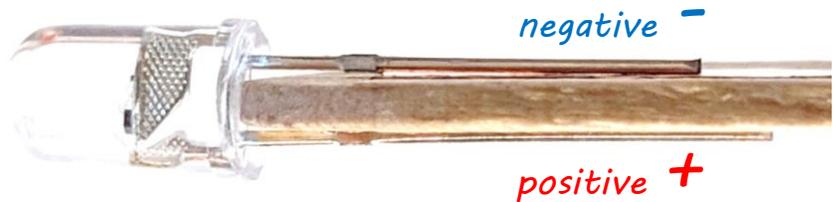
Cover the leads of the LED with copper tape. Rub or “burnish” the copper tape with the edge of your fingernail or the back of a pen/etc. to ensure a solid connection to the LED!
